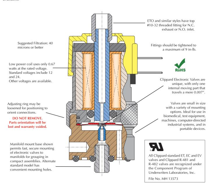
Clippard Minimatic electronic valves are precision-built 2-way or 3-way control valves, utilizing a unique, patented, valving principle. There are no sliding parts. Complete poppet travel is a mere 0.007". As a result, low power consumption and exceptionally long life are major benefits of this design.
